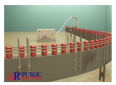
Republic Air Knife Systems are sized complete with accessories to insure no unexpected bends compromise drying results.
