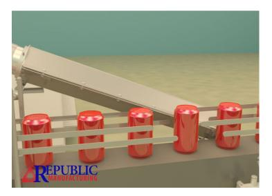
Republic recommends cutting rails so the airstream is uninterrupted to provide optimized drying results.
