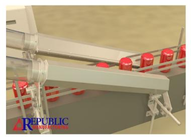
The angle of the air knives is key to insuring a completely dry can.
