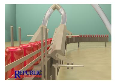
Republic Air Knives are strategically placed along the sides of the cans to shear water from the top to the bottom.
