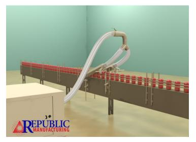
Republic manufactures manifolds such that one blower may power multiple air knives. Republic's Air Knife Brackets are fully adjustable and hold the air knives steady throughout the drying process.
