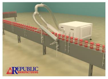
Air is piped through stainless steel tubing or PVC smooth bore hose to reduce friction, providing the ideal flow and pressure. Flex hose is available for sharp bends.
