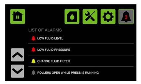
**Process monitoring -** The SmartFlow® controller can monitor pressure, flow, valve performance and line status to ensure lubrication is delivered as required
